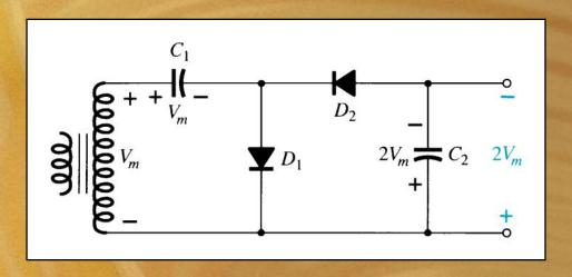
This half-wave voltage doubler's output can be calculated using:
